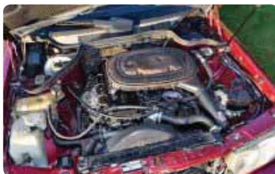
▽ The 2.3-litre, eight-valve M102 with 134bhp.
