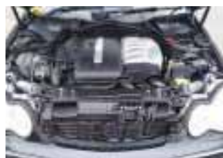
△ The 2,685cc five-pot in the C270 CDI makes 168bhp/295lb ft torque, and achieves 40mpg.
