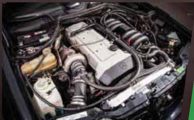
▷ Garrett T03 turbo fits neatly in the engine bay.
